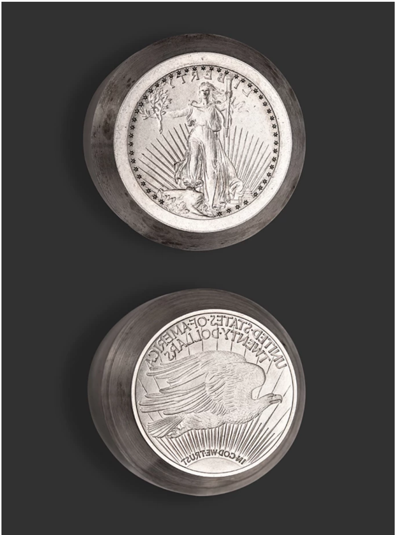
UNDATED DIES FOR THE LOW RELIEF VERSION OF THE SAINT-GAUDENS DESIGNED DOUBLE EAGLE. (PHOTO: UNITED STATES MINT)
